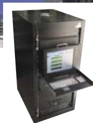
**RTMS-2001R:** This commercially-off-the-shelf system provides multi-channel, real-time data acquisition and analysis with manual and event-driven triggering. The system also offers an extensive set of remote tools for real time monitoring, broadcasting streaming data, data retrieval, remote tele-control, and event driven notification.
